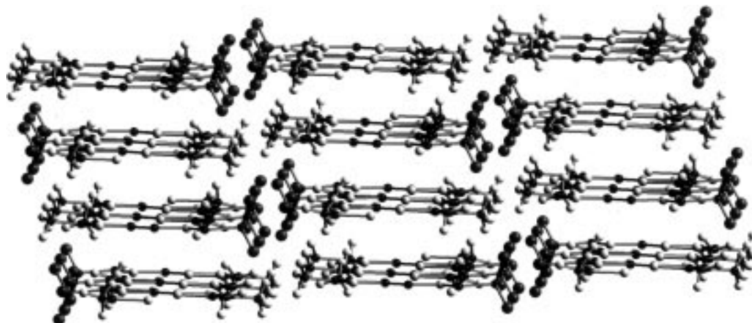
Figure 9. The layered, zwitterionic radical (\text{Me}_3\text{TTF}^+)\text{PO}_3\text{H}^- . The larger dark spheres represent the O atoms of the \text{PO}_3\text{H}^- substituents engaged in the hydrogen-bond network. 85
